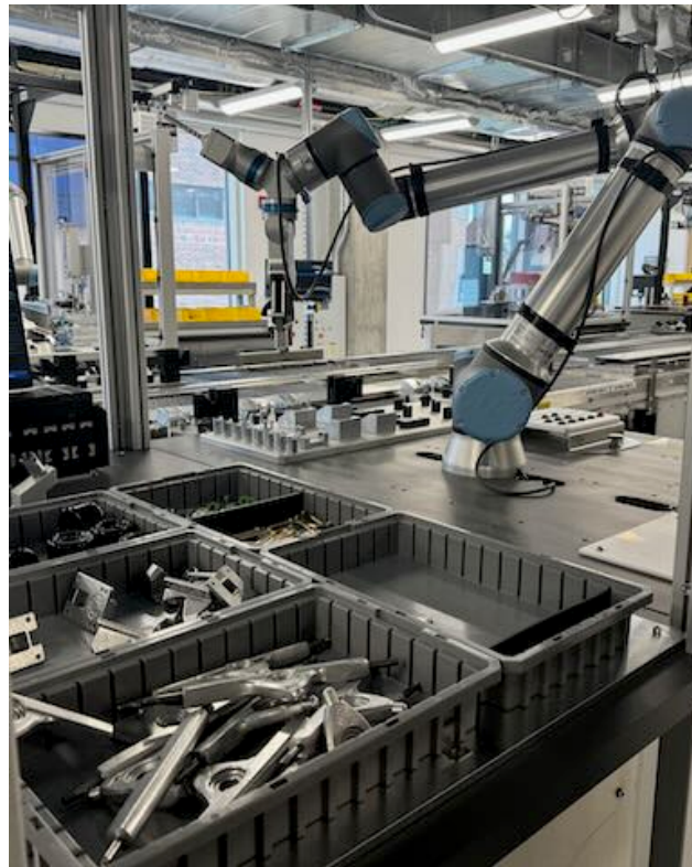
Figure xxx: Main assembly area of Smart Manufacturing facility at Purdue. There is a robot picking parts from bins to populate a set of fixtures for assembly.
