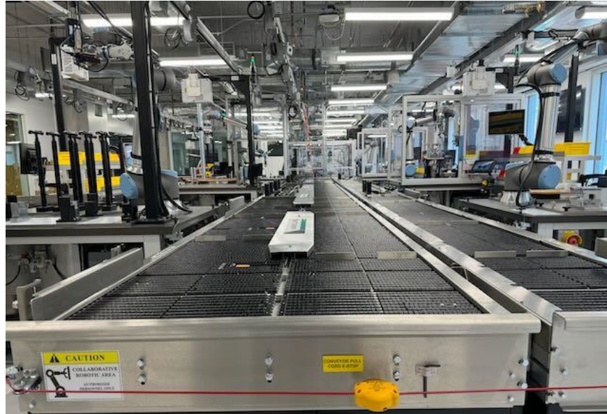
Figure xxx: Main assembly area of Smart Manufacturing facility at Purdue. There is a main conveyor system, side conveyor systems flanked by robots and associated fixturing
