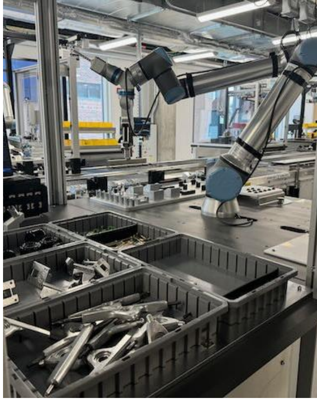
Figure xxx: Main assembly area of Smart Manufacturing facility at Purdue. There is a robot picking parts from bins to populate a set of fixtures for assembly.
